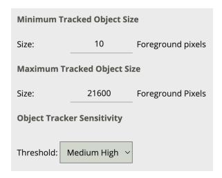
The motion based Object Tracker now support a Maximum Object Size as well as a Minimum Object Size. This allows for more control over which objects will be tracked by allowing the user to set an upper threshold that can remove large environmental issues that could cause false alarms.
