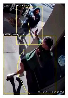
The Aggressive Behaviour rule is a detection algorithm that analyses the whole field of view over a set number of frames and estimates the likelihood that a fight is occurring. The algorithm is tracker independent and does not use the location of objects in the scene as an indicator of aggressive behaviour.
