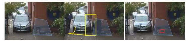
**Note:** The algorithm used for abandoned and removed object detection is the same in each case, and therefore cannot differentiate between objects which have been abandoned or removed. This is because the algorithm only analyses how blocks of pixels change over time with respect to a background model. **Note:** The algorithm used for abandoned and removed object will only work when the Object Tracker is selected under Trackers
