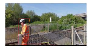
The previous image illustrates how the colour filter prevents objects, which do not contain the specified colours, from generating an event. In this case only the person generates an event but not the train line.
